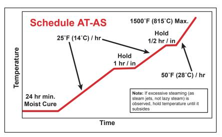
furnace/vessel such as weep holes, wicking and/or venting. Moisture driven and entrapped in the back up insulation is dangerous and may lead to spalls/explosions at elevated furnace temperatures. This is of special concern in floors/hearths.
