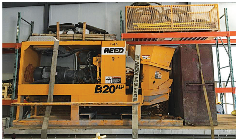
Pump used for PliShot Si-Bond B application.
